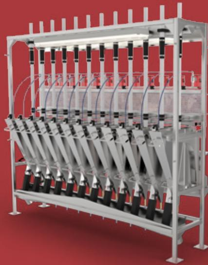
Our secondary sampling tanks are fully automatic and are used with both the Boxray 24 and Boxray Compact. In addition to the streams being screened and flowing down to the analyzer, daily average samples are collected. These daily samples flow down to special containers (pots) with perforated bottoms, where the water is drained from the samples, which makes work fast and effective for lab personnel.
